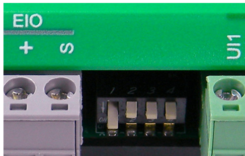
Illustration 1: CAN-590x expansion module address switches Illustration 2: Expansion module address switch positions
