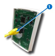
Plug an Ethernet patch cable 1 connected to an STE-9000 Series NetSensor into the (yellow) ROOM SENSOR port of the controller.
