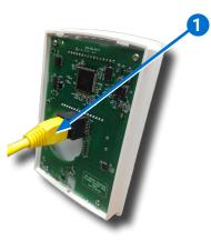
Plug an **Ethernet patch cable 1** connected to an **STE-9000 Series NetSensor** into the (yellow) **ROOM SENSOR port 2** of the controller.
