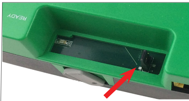
Watchdog Jumper on BAC-9001CE (Outside Cover)
