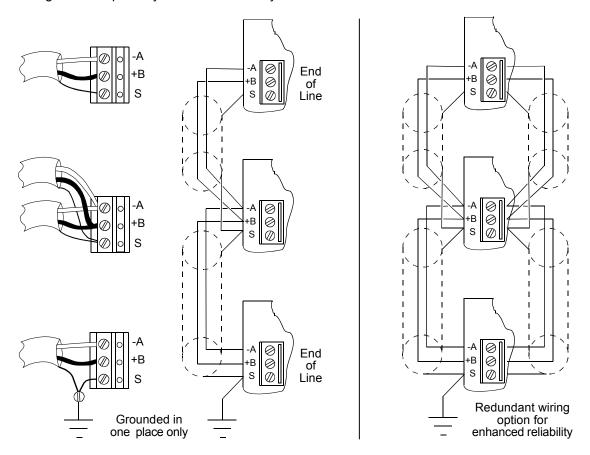
Figure 8: EIA-485 Network Wiring Details and Redundant Option
