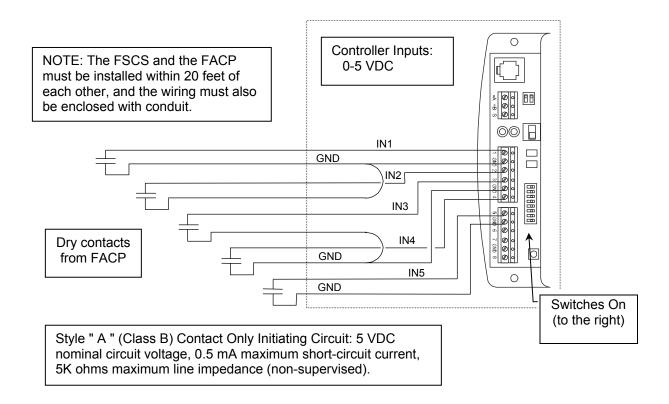
Figure 1: Sample Input Signals from the FACP
