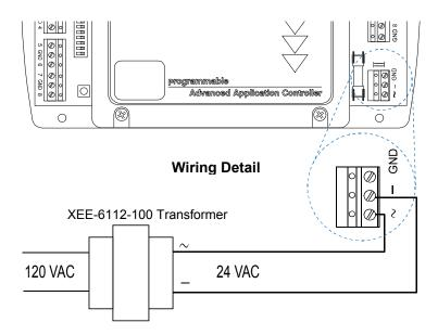
Figure 7: Installation and Power Wiring
