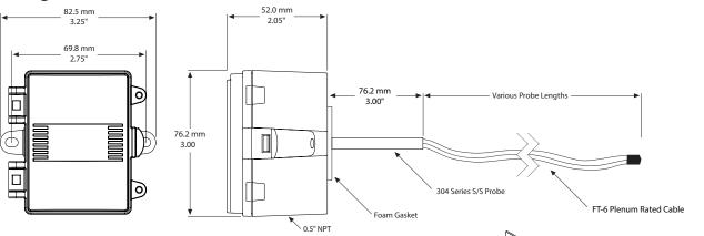
The averaging temperature sensor incorporates several discrete sensors encapsulated at equal distances across the length of the probe. The complete assembly acts as a single sensor to monitor the average temperature in a duct. (Averaging elements are not recommended for high humidity applications.)
