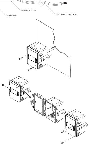
4. For the cable leading to the building automation system controller, attach conduit to the 1/2" NPT threaded connection hole that is provided in the bottom of the enclosure as needed.
