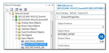
In default Conquest applications, **Al2 is mapped** to **AV2 (with a multiplier AV12) for the setpoint offset** 17, and AV2 is the value used in room temperature control programming (not Al2 directly). AV2 = Al2 x AV12.
