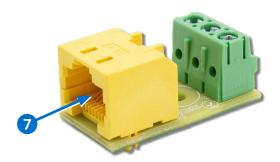
4. Plug the other end of the Ethernet cable into the ROOM SENSOR port 1 of the controller. (See Introduction on page 1.)
