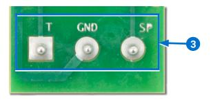
Connect wires from the thermistor to the Temperature 4 and Ground/Common 5 terminals on the adapter. (See Sample Wiring on page 2.)
