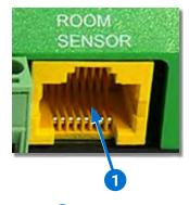
The **Room Sensor port 1** in KMC Conquest controllers is designed to automatically connect and configure a digital **STE-9000 Series NetSensor** or an **STE-6010**, **STE-6014**, or **STE-6017** analog (thermistor) sensor using a standard Ethernet patch cable.
