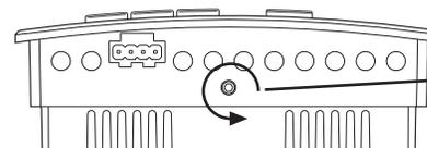
Turn counterclockwise until the screw engages the base.
