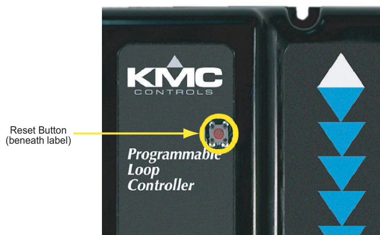
Illustration 10. Reset Jumper Detail
