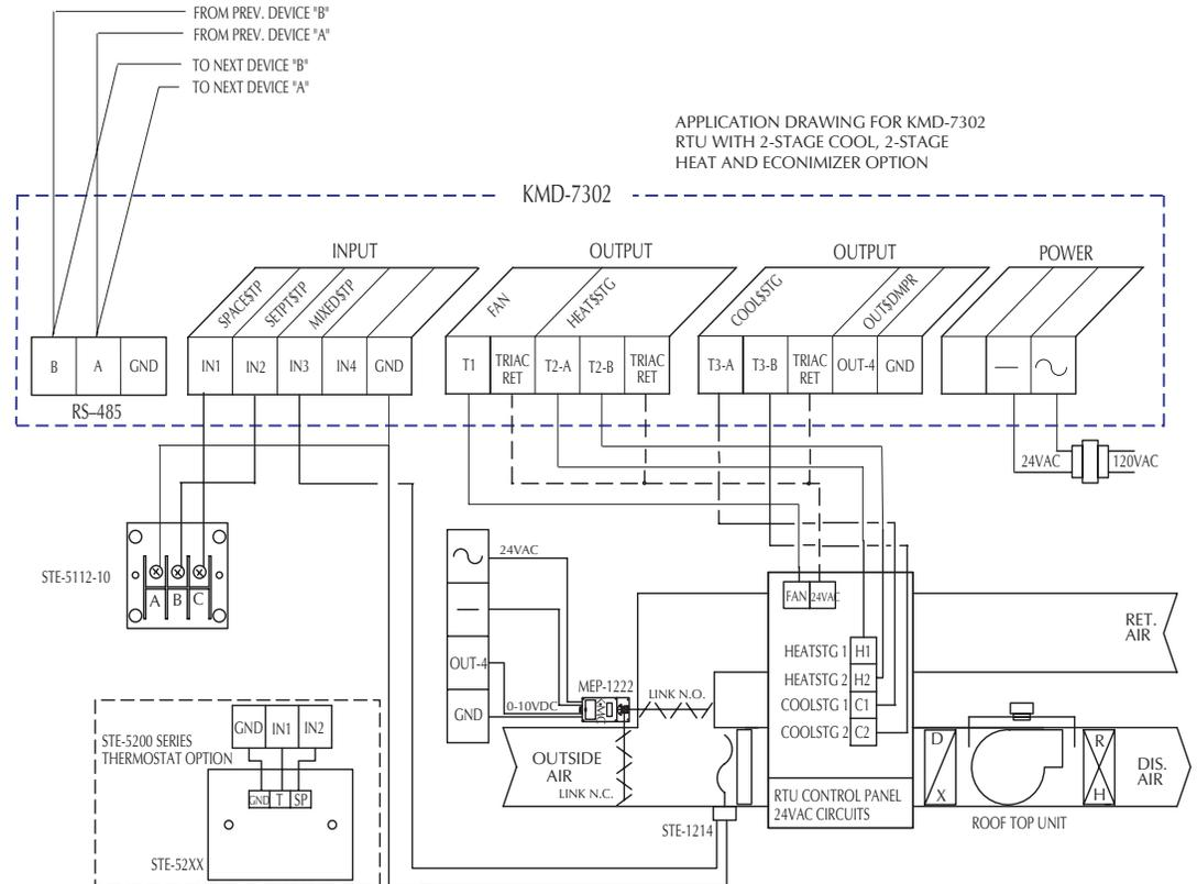
Illustration 6. Typical Controller Application Diagram
